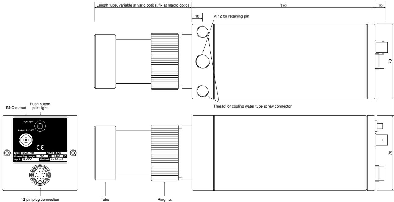
Figure 1: Drawing pyrometer
