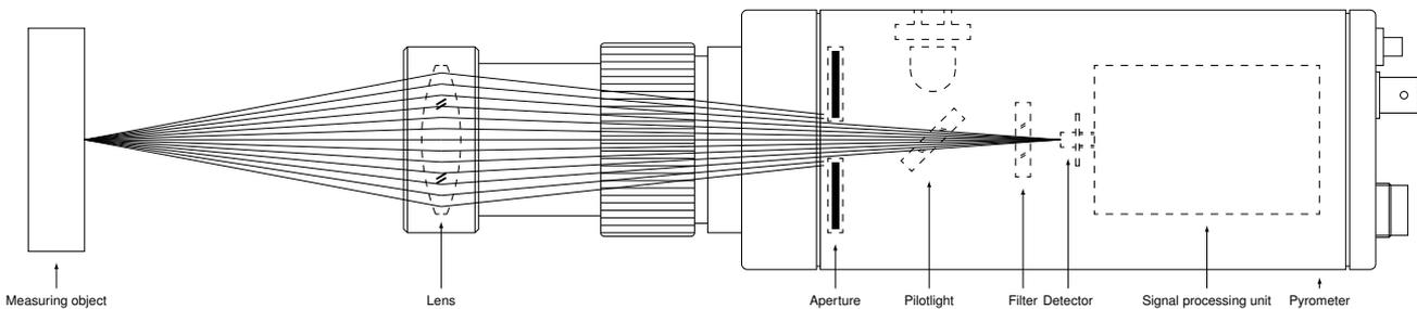
Figure 2: Structure of the pyrometer
